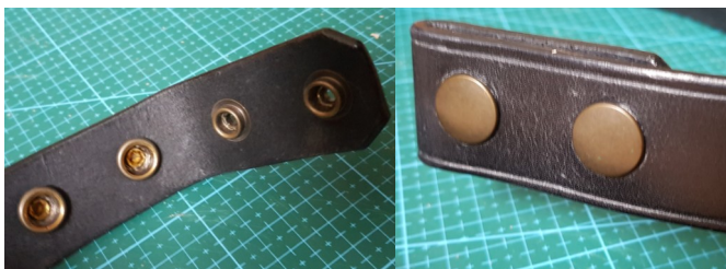
Press-studs on a buckle turn (for a Western-style buckle)
